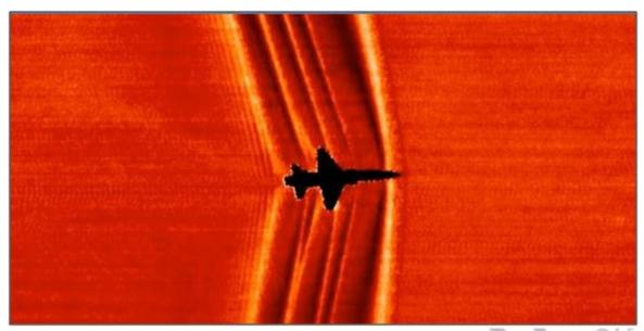
The shock wave forms a "cone" of pressurized or built-up air molecules, which move outward and rearward in all directions and extend all the way to the ground.
